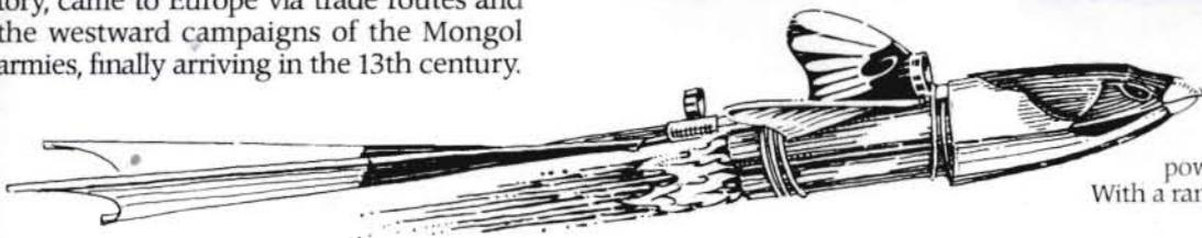
This bird bomb had a woven bamboo body packed with gunpowder. Four rockets protruded from its tail. With a range of 300 m, it could swoop down on an enemy, burning his camp or his ships.
